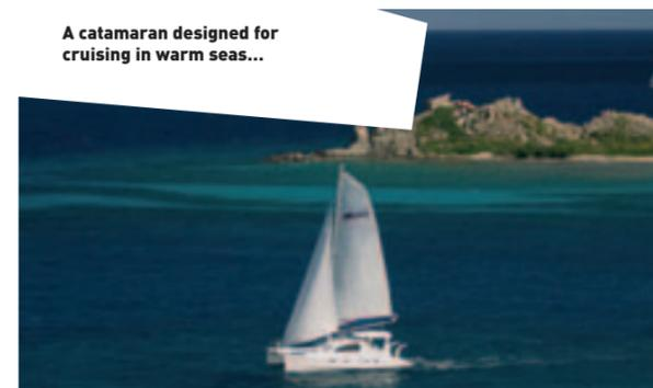
With two reefs in the main and 6 rolls in the genoa, the boat is well-balanced and sails easily at about ten knots.
